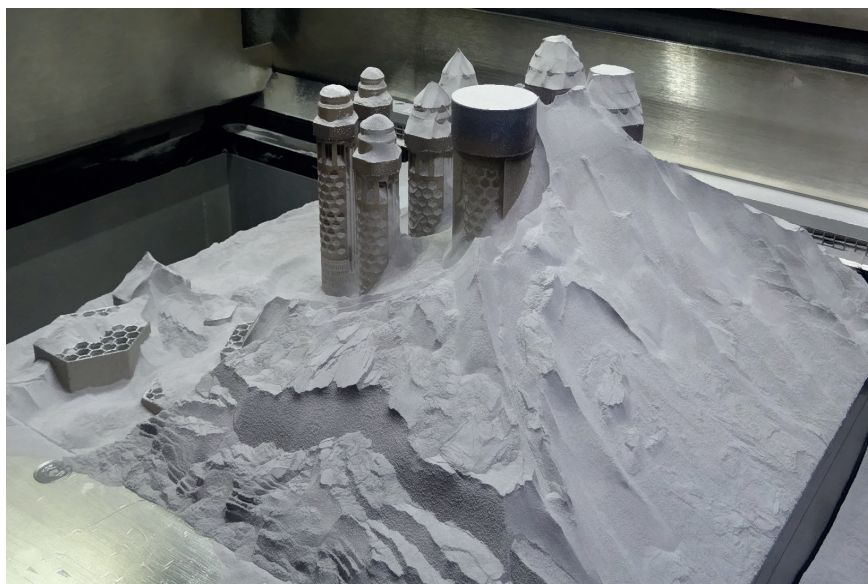
A mold-making job with up to 30 nozzles is processed in the SLM machine in about 24 hours.
